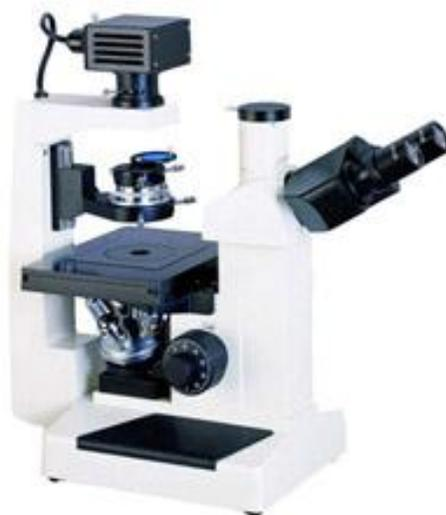
XDS-1 Inverted microscope is equipped with wide field eyepieces, long working distance plan achromatic objectives, long working distance condenser and phase contrast unit. It can be observed transparent and unfinished living specimen in culture bottle or culture utensil. It is the ideal instrument suitable for research of living specimen structure, liquid, deposits and so on. It also can be used in research institutes, universities, medical treatment, agriculture and animal husbandry etc.
